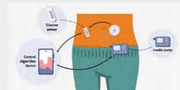
Schematic drawing of the components of the closed loop system
