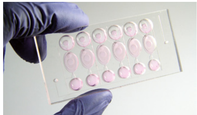
The lung-on-chip with 6 independent alveolar barrier systems filled with cell culture medium.
