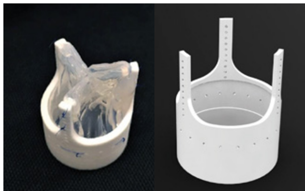
Printed valve holder with a biogenic polymer patch sutured inside (left), 3D-printed valve holder design (22mm) (right).
