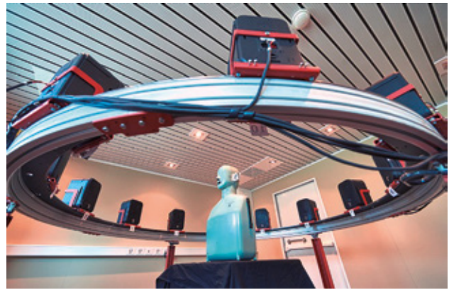
Multi speaker set up for sound field audiometry.
