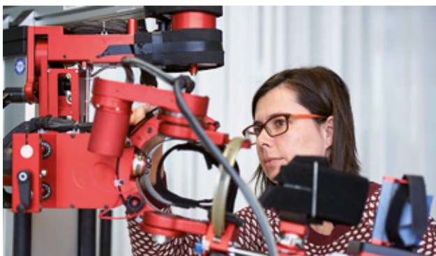
Developing new control strategies for upper limb rehabilitation robots.
