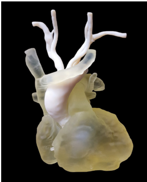
Construction of 3D-heart-models through rapid prototyping.
