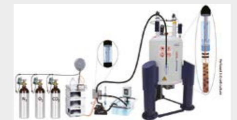
Bioreactor for online Metabolomics of living cells inside the NMR.
