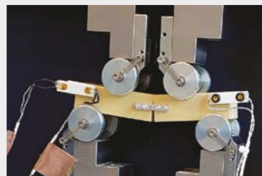
Mechanical test of osteosynthesis plates and screws
